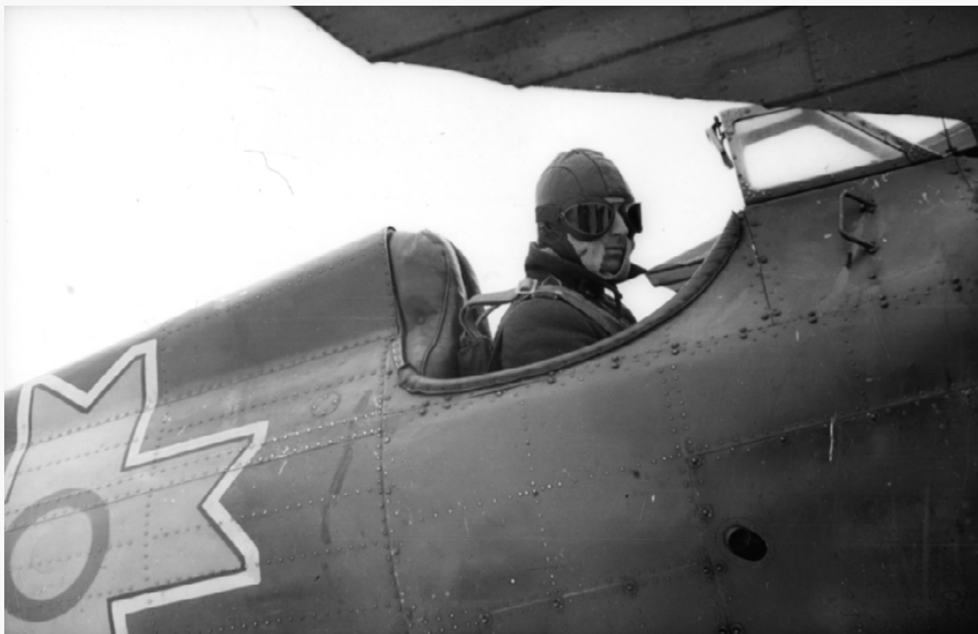
Close-up of the cockpit. Just behind the pilot's headrest a circular skin patch can be seen where the antenna insulator was previously fitted (the aircraft had no radio installed). Note the wear of the paintwork and the fact that the cross on the visible right side of the fuselage was slightly further back than on the left side. (Dan Antoniu/Horia Stoica collection)
