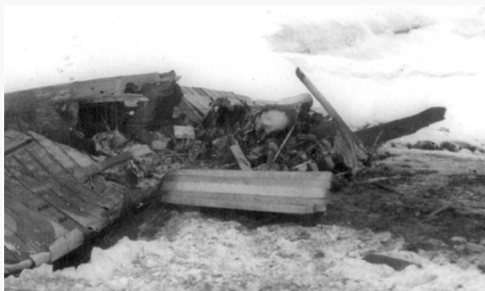
Two photographs of P.11F No. 83 wrecked in the winter of 1940/41. On the sides of the burnt-out fuselage there are visible wide skis without aerodynamic fairings, shod with three metal protective strips. The N-shaped truss is well visible. (Dan Antoniu/Horia Stoica collection)
