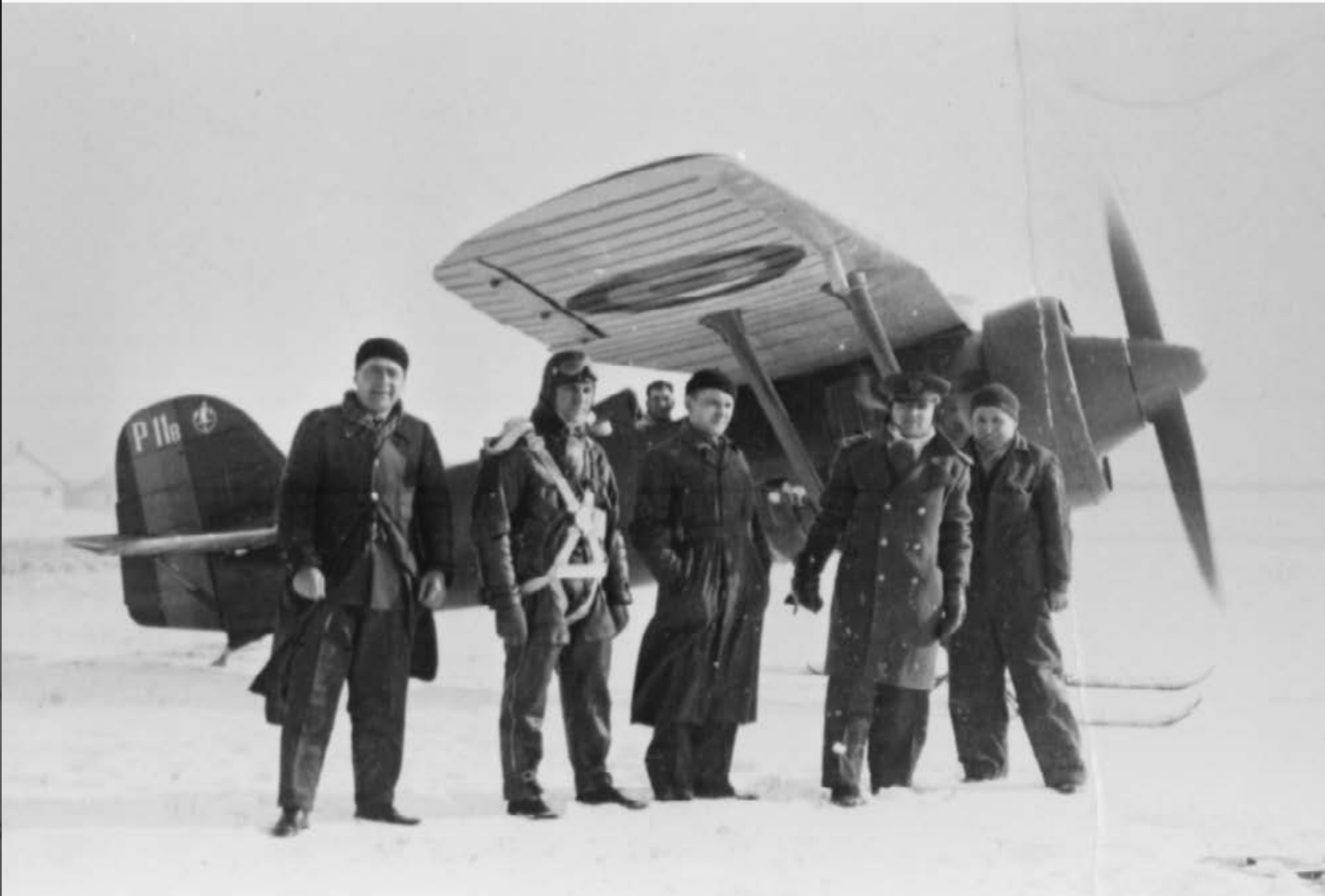
» Long, narrow skis of I.A.R. manufacture fitted to P.11B in the winter of 1936/37. (Dan Antoniu/Horia Stoica collection)
