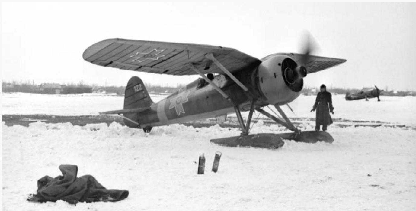
Last moments before take-off. In front of the aircraft two fire extinguishers can be seen. They were always kept on standby during engine start-up. This photo shows that, unlike the fuselage, the crosses on the lower surfaces of the wings had dots in the same colour as the cross rim. The aircraft had the armament removed, but the holes in the wings were not covered with plugs. Same as No. 128 this airplane has a small-bomb or grenade dispenser installed inside the wing (with a sliding cover). (Dan Antoniu/Horia Stoica collection)
